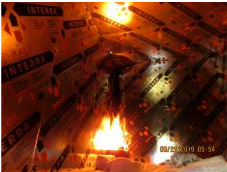
Photo No. 2 40KW fire exposure
