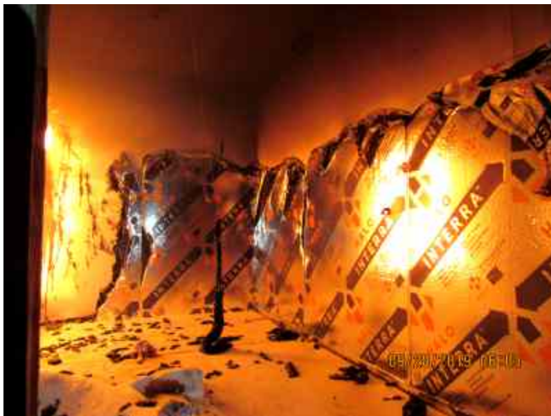
Photo No. 6 Foam consumption side wall opposite burner
