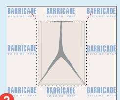
Make an inverted Y cut in the wrap at window rough opening. Make diagonal cuts at the top of the rough opening corners.
