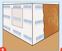
Start 2-3 feet from a corner. Wrap around corner and continue nailing or stapling as you move around the house. Use fasteners that are long enough to penetrate into the stud or nail base material.
